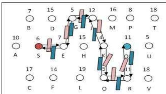
Figure 18. from Q to S ACK Packet is Forwarded
