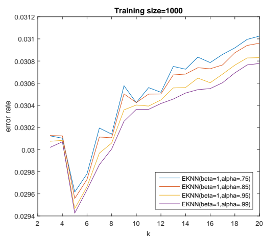
Figure 11. Plots of Mean Error Rates for EKNN for Different Values of \alpha with \beta=1 as a Function of k for Training Size 1000
