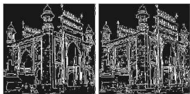
Figure 9. Edges obtained using Sobel method with 0.6 threshold value and Edges obtained using adaptive threshold
